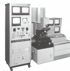
LSI photomask inspection system in 1976 (Winner of “Ten Best New Products Award” from Nikkan Kogyo Shimbum)
